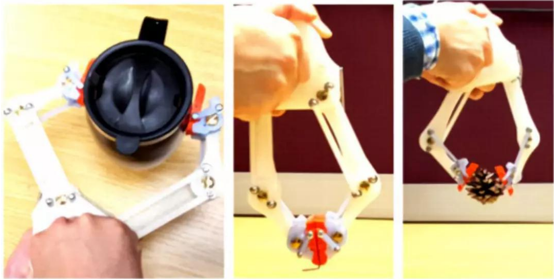
图 | 自适应机器人手 (来源 : Bai, G., Kong, X., & Ritchie, J. M. (2017). Kinematic Analysis and Dimensional Synthesis of a Meso-Gripper. Journal of Mechanisms and Robotics, 9(3), 031017. 4.)
